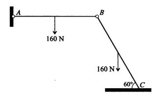
Two identical uniform rods, AB and BC, are freely jointed to each other at B, and A is freely jointed to a fixed point. The rods are in limiting equilibrium in a vertical plane, with C resting on a rough horizontal surface. AB is horizontal, and BC is inclined at  $60^{\circ}$  to the horizontal. The weight of each rod is 160 N (see diagram).
