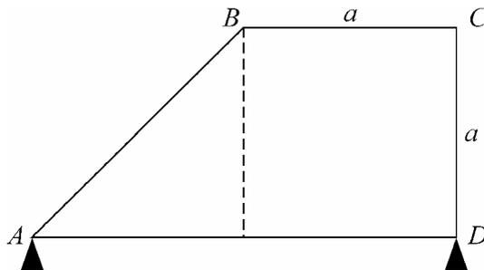
A uniform lamina  $ABCD$  has the shape of a square of side  $a$  adjoining a right-angled isosceles triangle whose equal sides are also of length  $a$ . The weight of the lamina is  $W$ . The lamina rests, in a vertical plane, on smooth supports at  $A$  and  $D$ , with  $AD$  horizontal (see diagram).
