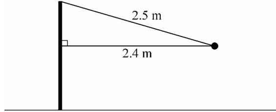
A ball of mass  $0.08 \text{ kg}$  is attached by two strings to a fixed vertical post. The strings have lengths  $2.5 \text{ m}$  and  $2.4 \text{ m}$ , as shown in the diagram. The ball moves in a horizontal circle, of radius  $2.4 \text{ m}$ , with constant speed  $v \text{ m s}^{-1}$ . Each string is taut and the lower string is horizontal. The modelling assumptions made are that both strings are light and inextensible, and that there is no air resistance.
