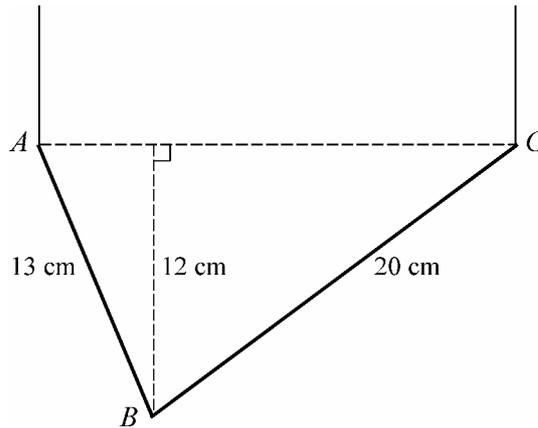
A rigid body  $ABC$  consists of two uniform rods  $AB$  and  $BC$ , rigidly joined at  $B$ . The lengths of  $AB$  and  $BC$  are 13 cm and 20 cm respectively, and their weights are 13 N and 20 N respectively. The distance of  $B$  from  $AC$  is 12 cm. The body hangs in equilibrium, with  $AC$  horizontal, from two vertical strings attached at  $A$  and  $C$ . Find the tension in each string. [8]
