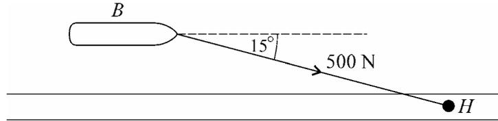
A barge  $B$  is pulled along a canal by a horse  $H$ , which is on the tow-path. The barge and the horse move in parallel straight lines and the tow-rope makes a constant angle of  $15^\circ$  with the direction of motion (see diagram). The tow-rope remains taut and horizontal, and has a constant tension of 500 N.
